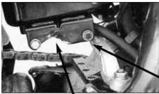
Cut a notch in oil tank support bracket as pictured above for clearance on the back side of the starter
