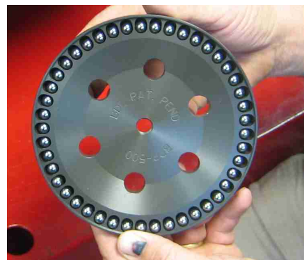
BPP-500 Lock up for HD 1998-2007 BDL pressure plate with 45- 5/16" chromium steel ball bearings. Install with stock HD diaphragm, retainer and bolts and install as per HD manuel. Re-adjust clutch as per HD manuel.
