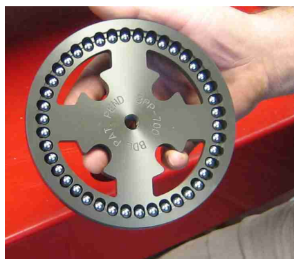
BPP-700 Lock up for Primo belt drives 1990-2007. Pressure plate with 42-5/16 " chromium steel ball bearings.
