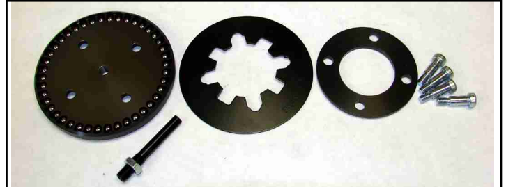
BDL Ball Bearing pressure plate with special diaphragm, retainer and new CDAS-500 adjusting screw
